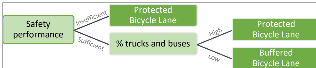
Figure E-3: Domain B Flowchart – Low vehicular speed and high traffic volume
